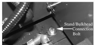
Figure 2-6. Bolt Connecting Stand to Bulkhead
