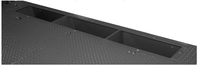
Figure 5-1. End Cleanouts with bolts and cover plate removed
