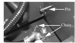
Figure 2-7. Hitch Pin and Chain
