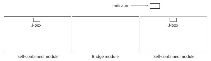
Figure 2-1. Module Placement
