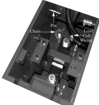
Figure 2-9. Load Cell Cover Plate Removed
