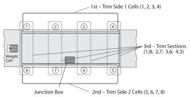
Figure 4-1. Load Cell Trimming Diagram
